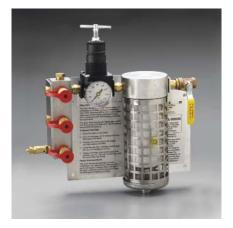
This panel is designed to filter and regulate air being delivered to the supplied air respirator. It has a maximum capacity of 50 cfm at 105 psig. This is an economical system that provides single step filtration. It is designed to be permanently mounted to the wall. It provides a maximum of 50 cfm to 3-5 outlets.
